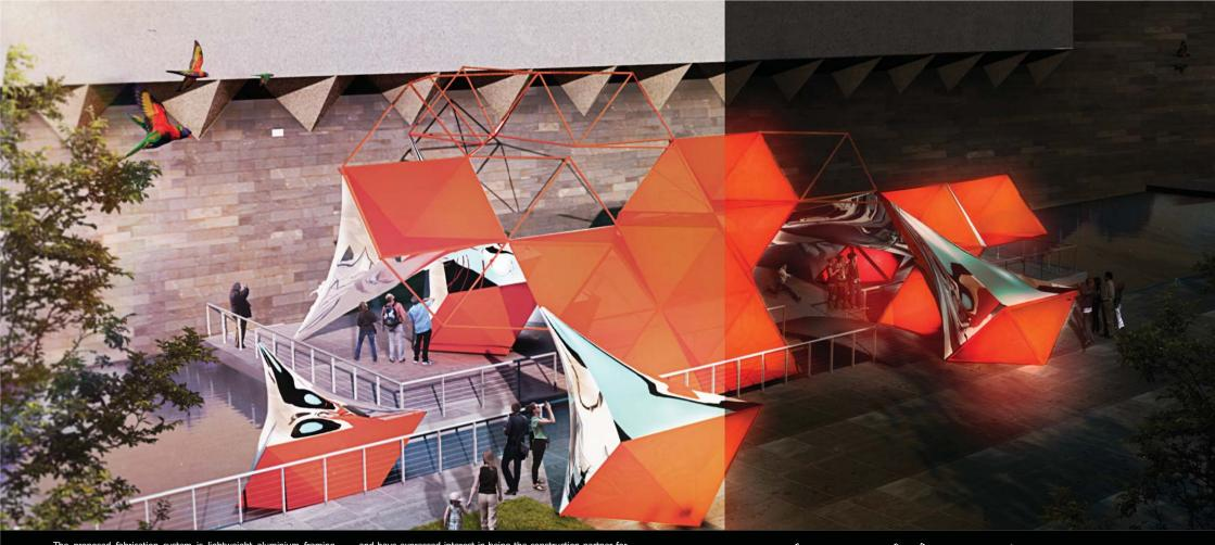
The proposed fabrication system is lightweight aluminium framing with coloured non-flammable PVC skins which are tightened under the effect of heat. Innovative fabrication company Barrisol Ryan Australia has reviewed the constructability and suitability of the system to the location, six-month time-frame as well as providing a budget estimate,
